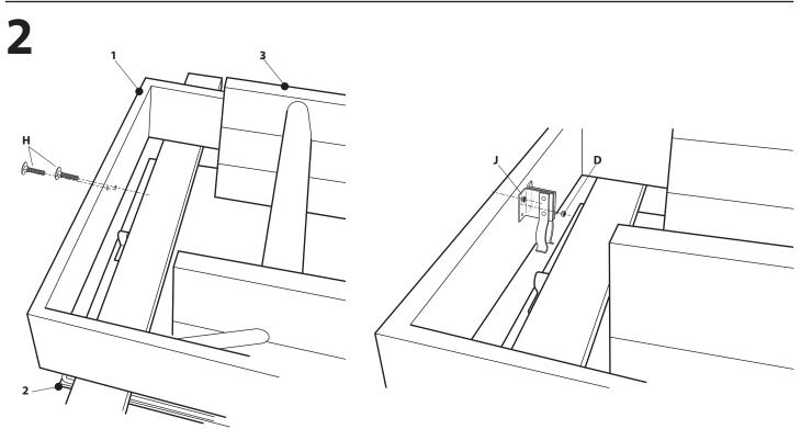
Use a hammer to tap coachbolts 'H' into position. Place part 1 on top of base board 3 separated by an off-cut of wood
